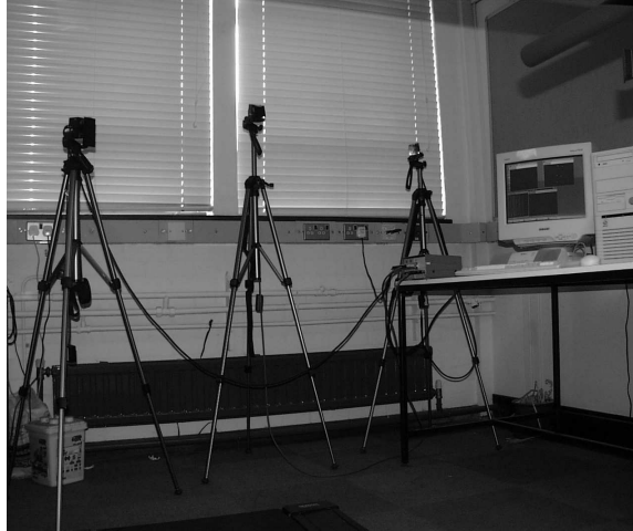
FIGURE 1.1. 3-camera motion capture system
